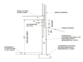
ALTERNATE FOUNDATION WALL/BRICK DROP SECTION
